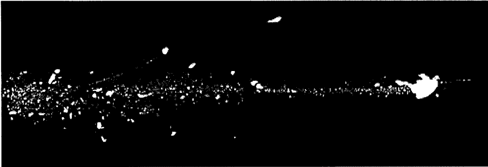
Lead bullet fragmentation upon entry into ballistics gel
